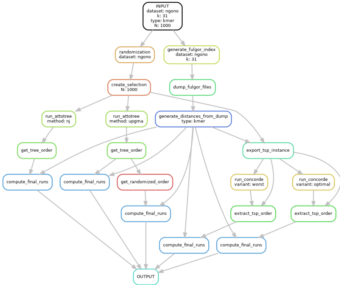
Figure 4.1: Example directed acyclic graph of the evaluation pipeline. This diagram shows the Snakemake workflow for a single dataset ( ngono ), a single k -mer size ( k = 31 ), one matrix type ( k -mer), and one dataset size ( N = 1000 ). The graph illustrates the rules for genome selection, Fulgor index construction, unitig and color-set extraction, Hamming distance computation, TSP instance generation and solving, phylogenetic tree inference via Attotree, and final RLE run evaluation across multiple ordering strategies. Although this example omits other datasets and parameter combinations for simplicity, the implemented workflow generalizes to all configurations used in the experiments.
